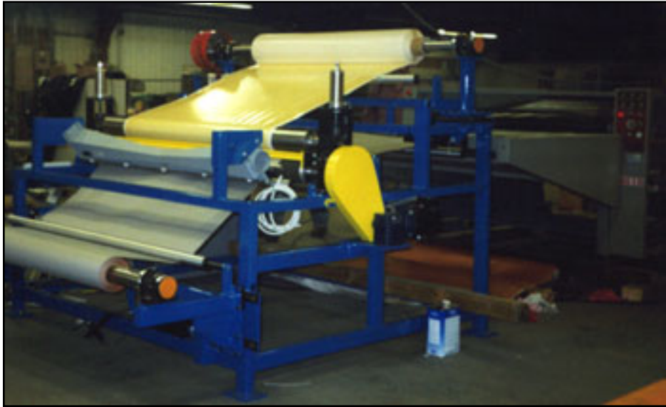
Two position Unwind Stand and Driven Pull Roll to strip release paper from adhesive before entry into Astex 6800 Laminator
